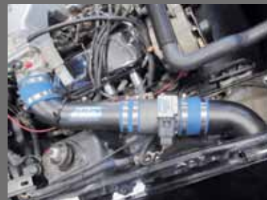
During our normally aspirated runs a BBK cold-air intake provided the lungs for the dyno. The black finish looked great under the hood and it produced a wicked intake honk under WOT.
