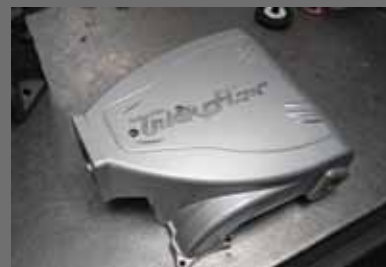
A Trick Flow Street Burner intake manifold topped our stroker motor and kept us legal with the smog enforcers. The long-runner design is good for big torque down low long before boost rolls in.
