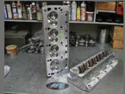
Behold the all-new AFR Renegade 195 emissions-legal heads that flow a massive 317 cfm at 0.650 lift. They not only have solid low- and mid-lift numbers, but they out flow the outgoing 205cc models.
