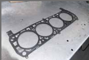
Fel-Pro PermaTorque 1133 MLS head gaskets ain't cheap, but they're beyond strong and a must for any forced-induction build. Again, spend a little more up front to save it in the long run since replacing blown head gaskets is PITA.
