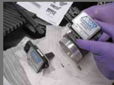
The 76mm BBK MAF allowed us to swap MAF cards for both the 30-pound and 42-pound injectors. It's important to spec your MAF to your injectors or your car will never run correctly.
