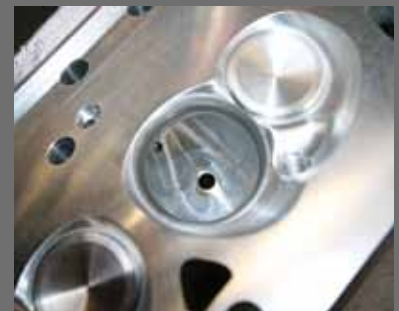
The 195s feature full factory-CNC ported runners and combustion chambers. See inside—that's the kind of quality we've come to expect from AFR. The valves measure 2.05-inch intake and 1.60-inch
