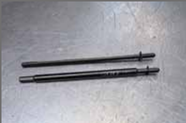
It's the small things that go a long way and adding pieces like an ARP oil-pump shaft is key to a pumped-up engine's longevity. Note how much bigger it is than the stock unit.
