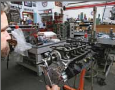
Rankin Performance Machine was commissioned to assemble the motor since quality parts mean nothing without a proper installation. Here John Rankin is dialing in the Ford Motorsports timing cover. Without the proper alignment, the front bearings will quickly burn up.
