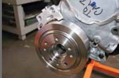
A Summit Racing Supercharger-spec harmonic balancer was the perfect 28-ounce addition to the motor, along with a Ford Racing Performance Parts timing pointer. Note that a spacer must be used to mate the balancer to the Fox-body accessory drives; we used an FRPP unit (Summit PN FMS-M-8510-B351).
