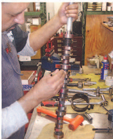
▲ There's a bit of trickery happening with the Clevor's cam. While we're using a Trick Flow Stage III hydraulic-roller piece (0.574-inch-intake/0.595-inch-exhaust lift and 236/248 degrees duration at 0.050-inch) for this engine, a rocker-arm change (from 1.6 ratio) changes the cam's lift measurements dramatically. Details on that change are a few photos away.
