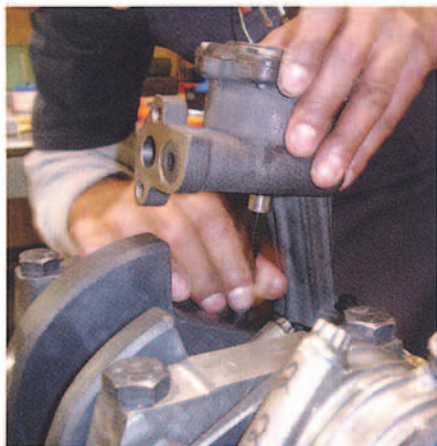
▲ The 351W's oiling system is much better than that of its Cleveland counterpart, which is one of the reasons a Clevor is a best-of-both-worlds engine package. Naturally, our intent is to keep oil flowing smoothly throughout the engine, so Melling's high-volume pump (PN 10833; $55.95) was chosen for the task. The stock-style pump features a larger inlet bore and hardened-steel gears, which help supply 25 percent additional oil flow. The pump's drive and idler shafts also have been extended into the cover to provide extra support.
