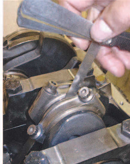
▲ Side clearance for each connecting rod is another internal-engine spec that should be checked (and oftentimes isn't). Only 0.025-inch separates the big ends of each rod in our bullet. The ARP rod bolts receive 65 lb-ft of torque.
