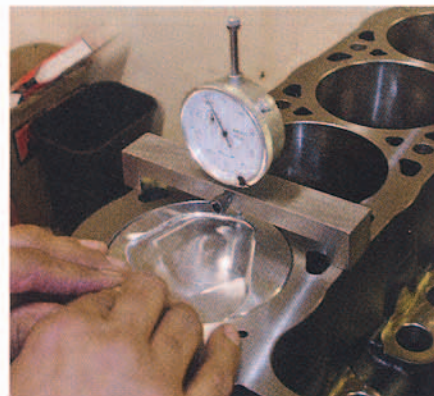
▲ We certainly don't want to experience any conflict between the pistons and the valves in our Clevor's Trick Flow PowerPort 225 cylinder heads. To ensure there is sufficient clearance, Tony uses a dial indicator to check piston deck height, which measures 0.008-inch from the top of the piston to the deck surface.
