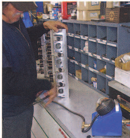
▲ Prior to installing cylinder heads, our engine's top-half assembler, Gary Guerrero, checks the valve seal on the new Trick Flow heads. Gary uses a vacuum tester for this procedure, which pulls 28 inches of vacuum at each port.
