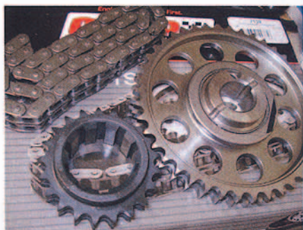
▲ The engine's valvetrain harmonics and total amount of deflection will be minimal thanks to this billet-steel roller timing set from Comp Cams (PN 7138; $89). The cam gear operates smoothly thanks to a Torrington bearing, and the set features a nine-position crank sprocket for 2-degree-increment adjustability and 8-degree-maximum advance/retard.
