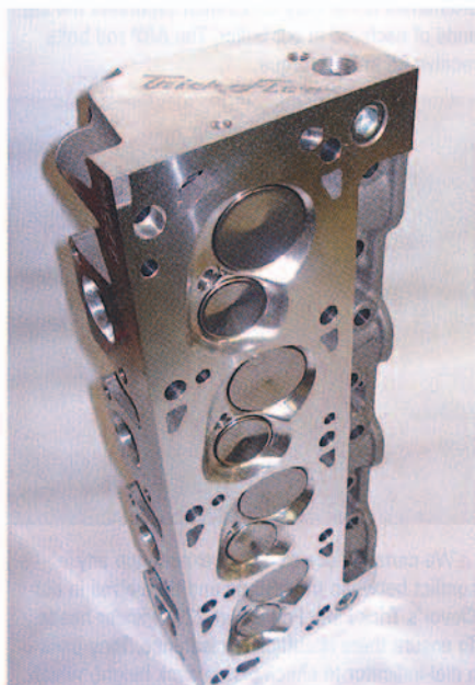
▲ Check the deck of Trick Flow's PowerPort Cleveland 225 aluminum cylinder head (PN TFS-5160T005-C01; $2,749.95). The fully assembled, CNC-ported heads feature 60cc combustion chambers, and stainless-steel 2.08-inch (intake)/1.60-inch (exhaust) valves. Notice the plug in the water passage on the head's deck surface and a new, threaded hole in the face of the cylinder head. These modifications are necessary for installing any 351 Cleveland heads on a Windsor-style block.
