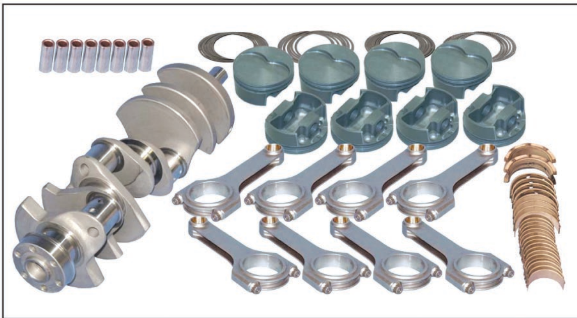
^ Eagle's competition 408ci 351W kit includes an Eagle forged 4340 steel crankshaft with 4.000-inch stroke, Eagle forged 4340 steel H-beam rods in 6.250-inch length, Mahle forged 4032 aluminum pistons and with various compression ratios and bore sizes available, Mahle plasma-moly file-fit rings, and Clevite H-series race bearings.
