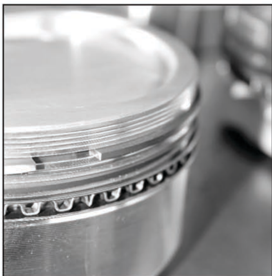
^ For piston rings, Coast used Clevite Perfect Circle pre-fit steel rings in the standard 1/16-inch top, 1/16-inch second and 3/16-inch oil ring sizes. The top ring is gap is .021-inches and the second ring gap is .024-inches.
