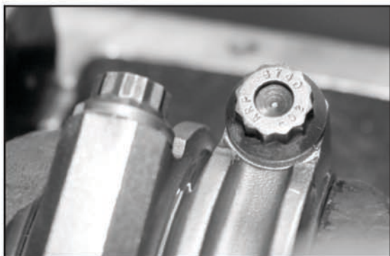
^ Attaching the rod cap to the connecting rod itself are ARP 7/16-inch 12-point rod bolts. There's no point in using quality parts if you aren't going to use quality fasteners to button everything up. Thankfully, ARP makes some killer fasteners to help everything stay together under serious loads.
