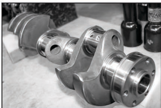
^ The foundation of any good rotating assembly is a good crank. Coast High Performance's 363 rotating assembly calls for a 3.400-inch stroke Probe crank. Forged out of 4340 steel, it features standard 2.248-inch main journals and 2.123-inch rod journals and should support our power goals, and then some.
